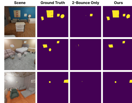
Fig. 14. Two-Bounce Only Ablation. We compare specular segmentation for models trained with transients rendered with only 1- and 2-Bounce peaks vs all peaks (ours). We randomly set pictures to be specular and find that only using 2-bounce information is not sufficient – thus, we posit this model also relies on 3-bounce information.
